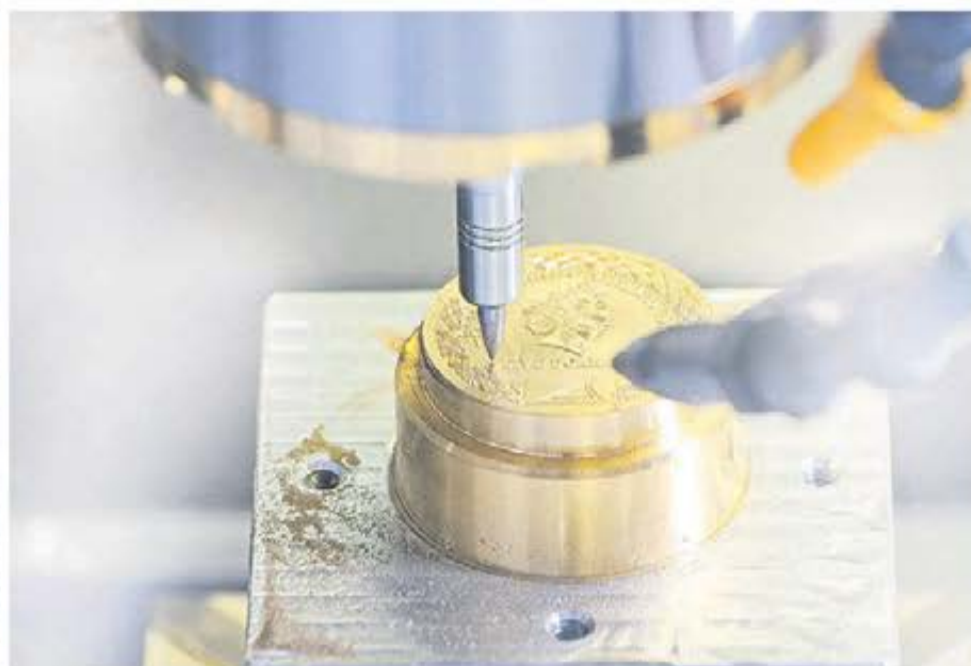
The combination of the air bearing spindles and ultra-fine balanced SCHUNK TRIBOS polygonal toolholders provides for im-mediate brilliant results in the production of coin punches.
