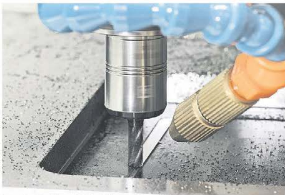
In mold making, the combination of ultra-precision machining centers and SCHUNK TRIBOS polygonal toolholders achieve per-fect surfaces.
