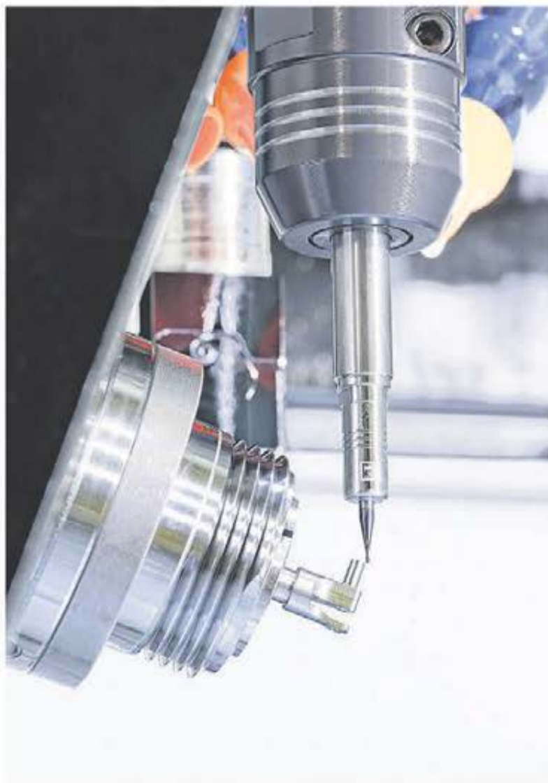
For the production of medical instruments, this application combines SCHUNK TENDO E compact hydraulic expansion tool-holders with SCHUNK TRIBOS extensions.
