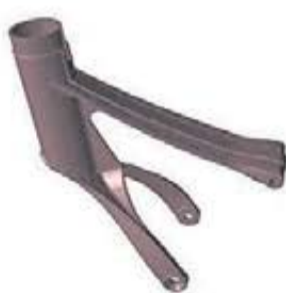
1. CAD model of seat post designed for aluminium alloy casting
