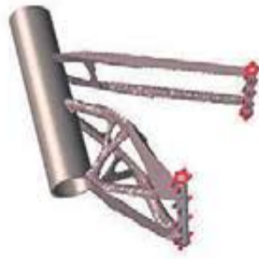
2. Topological optimisation using Altair's solidThinking Inspire® 9.5 software
